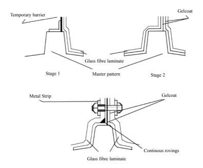
150mm or so, to hold the two halves of the mould together.
