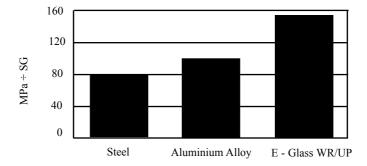
Figure 3 - Specific Tensile Modulus - Steel, Aluminium and GFRP
