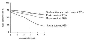
Figure 13 - Effect of weathering on the gloss retention of low fire hazard GFRP laminates with gelcoats
