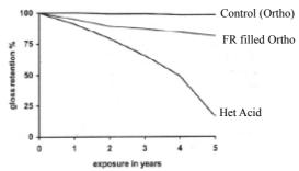
Figure 14 - Effect of weathering on the gloss retention of GFRP laminates with various surfaces (Orthophthalic resin/glass mat; 70% resin content)
