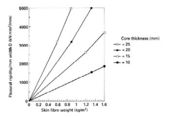
Figure 9 - The effect of WR (glass) skin construction (at R:F 1:1) and core thickness on flexural rigidity for balanced double skinned sandwich laminates
